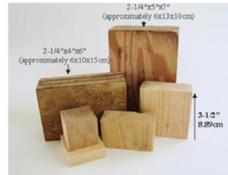
▲ You will need a variety of wood blocks to assemble the sconce. One block must measure 3-1/2" (8.89cm) either in length or height. It is used as a support when adding the front panel. The two largest blocks pictured here were made by gluing together 3 pieces of 3/4" (2cm) plywood which was then cut into blocks.
