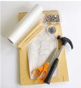
▲ To construct the jig you will need: A copy of the pattern; clear adhesive back vinyl, slightly larger than the pattern; a board to assemble the panel on; trim moulding; small nails; push pins; scissors and a hammer.
